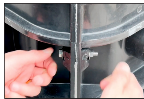
outside corners: bolt together - 3 per corner*
