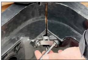
inside top corner: insert lid nut & corner brace*
